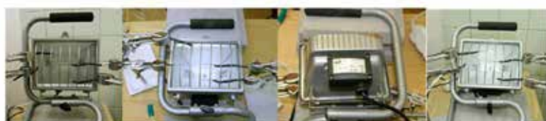
Svítlidlo REX 220-240 V~, 50 Hz, R7s max. 500W, IP 20, D 1m, halogenová žárovka: ECO HALOGEN XQ lite (XQ 0917), R7s/118 mm, 350 W, 230 V~, 50 Hz, 2900 K warm white, 7100 lm
